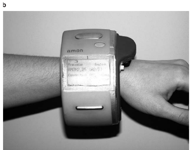
Figure 2 AMON prototype, mounted on the wrist, positions of sensors are shown. An SpO 2 sensor and thermopile are integrated into the cuff. (a) Cross-section of the first prototype and (b) picture of the second prototype.
